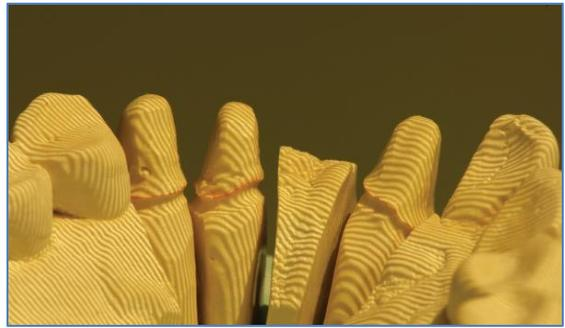
Fig 1: White light projector pattern during the scanning procedure by an optical scanner
